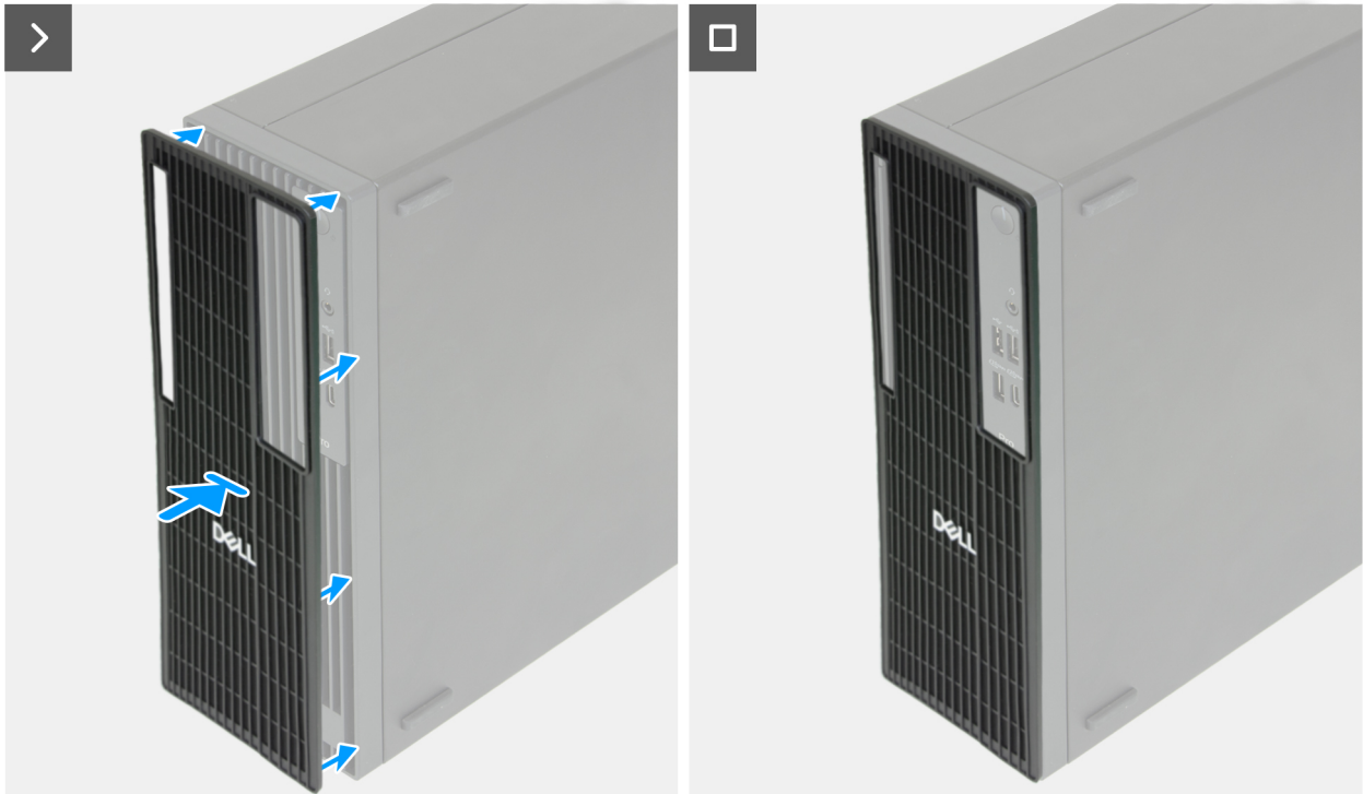
Figure 15. Installing the dust filter
